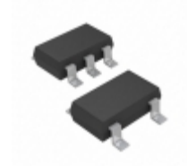
MIC5306-3.1YD5-TR Microchip Technology IC REG LDO 3.1V 0.15A TSOT23-5
