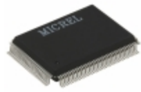
KSZ8995XA Microchip Technology IC SWITCH 10/100 5PORT 128QFP
