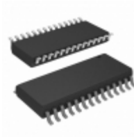
AT28HC256F-12SA Microchip Technology IC EEPROM 256KBIT 120NS 28SOIC
