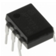
APT1212AX Panasonic Electric Works OPTOISOLATOR 5KV TRIAC 6DIP
