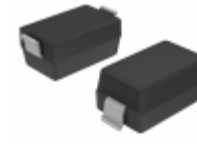
BZT52C43-E3-08 Vishay Semiconductor Diodes Division DIODE ZENER 43V 410MW SOD123
