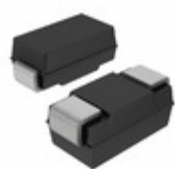
PTZTE2520B Rohm Semiconductor DIODE ZENER 20.8V 1W PMDS
