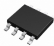
BR24G32FVM-3AGTTR Rohm Semiconductor IC EEPROM 32KBIT 1MHZ 8MSOP
