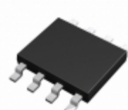
BR24G32FVJ-3GTE2 Rohm Semiconductor IC EEPROM 32KBIT 400KHZ 8TSSOP
