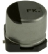
EEV-FK1C680P Panasonic Electronic Components CAP ALUM 68UF 20% 16V SMD
