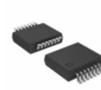
74LVT125DB,112 Nexperia USA Inc. IC BUFF TRI-ST QD N-INV 14SSOP
