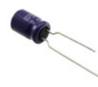
ECA-2GM2R2B Panasonic Electronic Components CAP ALUM 2.2UF 20% 400V RADIAL
