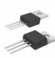
IXFP90N20X3 IXYS Corporation 200V/90A ULTRA JUNCTION X3-CLASS
