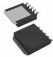
BD3570YHFP-MTR LAPIS Semiconductor IC REG LINEAR 3.3V 500MA HRP5
