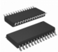
ICL3243CA Intersil IC 3DRVR/5RCVR RS232 3V 28-SSOP
