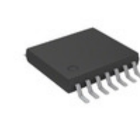
PIC16F684T-I/ST Microchip Technology IC MCU 8BIT 3.5KB FLASH 14TSSOP
