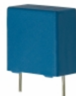
B32913A4334M EPCOS (TDK) CAP FILM 0.33UF 20% 440VAC RAD
