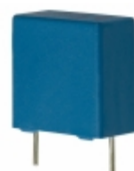
B32913A4334M000 EPCOS CAP FILM 0.33UF 20% 440VAC RAD
