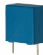
B32913A4104M000 EPCOS CAP FILM 0.1UF 20% 440VAC RADIAL
