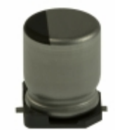
EEE-1HA470UP Panasonic Electronic Components CAP ALUM 47UF 20% 50V SMD
