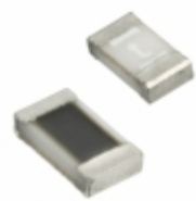
RR0816P-5760-D-74A Susumu RES SMD 576 OHM 0.5% 1/16W 0603
