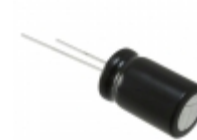
EEU-HD1E222 Panasonic Electronic Components CAP ALUM 2200UF 20% 25V RADIAL
