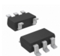
24AA02E48T-I/OT Microchip Technology IC EEPROM 2KBIT 400KHZ SOT23-5
