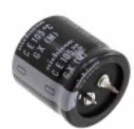
LGX2D681MELB30 Nichicon CAP ALUM 680UF 20% 200V SNAP
