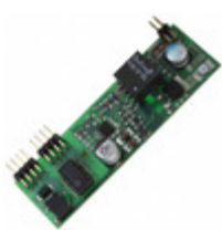
SPDCPOE05 STMicroelectronics MODULE POE 10W
