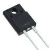
SRAF850 C0G TSC (Taiwan Semiconductor) DIODE SCHOTTKY 50V 8A ITO220AC
