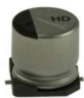
EEE-HD2A100P Panasonic Electronic Components CAP ALUM 10UF 20% 100V SMD
