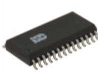
ISD2560SY Nuvoton Technology Corporation of America IC MEM VOICE REC/PLAY 60S 28SOIC
