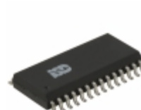
ISD2560SYR Nuvoton Technology Corporation of America IC MEM VOICE REC/PLAY 60S 28SOIC
