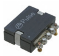
PA1393.352NL Pulse Electronics Corporation FIXED IND 3.5UH 12A 1.43 MOHM
