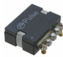
PA1393.302NLT Pulse Electronics Corporation FIXED IND 3UH 15A 1.43 MOHM SMD
