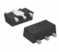
S-1137B28-U5T1G SII Semiconductor Corporation IC REG LINEAR 2.8V 0.3A SOT89-5
