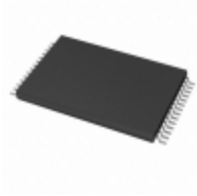
AT29LV256-20TI Microchip Technology IC FLASH 256KBIT 200NS 28TSOP
