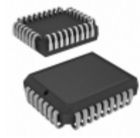
AT29LV256-20JI Microchip Technology IC FLASH 256KBIT 200NS 32PLCC
