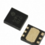
XC6121C522ER-G Torex Semiconductor Ltd IC WATCHDOG TIMER 6-USP
