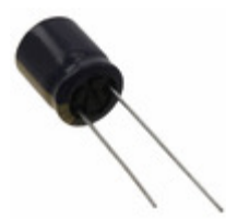
EEU-FC1C122B Panasonic Electronic Components CAP ALUM 1200UF 20% 16V RADIAL
