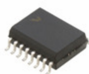
MC908QY4MDWER NXP USA Inc. IC MCU 8BIT 4KB FLASH 16SOIC
