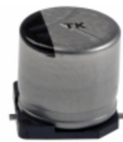
EEE-TKH681UAM Panasonic Electronic Components CAP ALUM 680UF 20% 50V SMD
