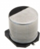
EEE-TP1A331AP Panasonic Electronic Components CAP ALUM 330UF 20% 10V SMD
