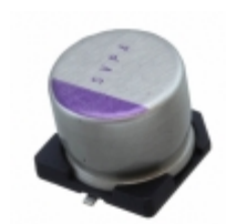
16SVP82MAA Panasonic Electronic Components CAP ALUM POLY 82UF 20% 16V SMD
