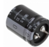
LGY1H332MELA30 Nichicon CAP ALUM 3300UF 20% 50V SNAP
