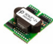
2SC0108T2D0-12 Power Integrations IC DUAL GATE DRIVER 8A
