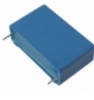
B32676G8475K000 EPCOS CAP FILM 4.7UF 10% 875VDC RADIAL
