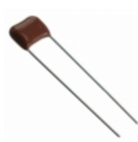
ECQ-E2153KFB Panasonic Electronic Components CAP FILM 0.015UF 10% 250VDC RAD
