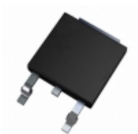
IXTY15N20T IXYS MOSFET N-CH 200V 15A TO-252
