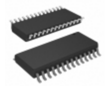
PIC16LF722AT-I/SO Microchip Technology IC MCU 8BIT 3.5KB FLASH 28SOIC
