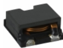
CEP125-0R3NC-UD Sumida America Components Inc. FIXED IND 350NH 18.5A 1.5 MOHM
