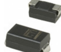
P4SMA36CA Littelfuse Inc. TVS DIODE 30.8VWM 49.9VC SMD
