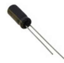
EEU-FC1C680B Panasonic Electronic Components CAP ALUM 68UF 20% 16V RADIAL
