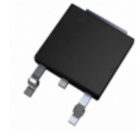
L78M08ACDT STMicroelectronics IC REG LDO 8V 0.5A DPAK
