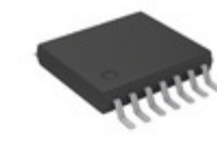
MCP4251T-104E/ST Microchip Technology IC DGTL POT 100K 2CH 14TSSOP
