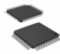
PIC16F877A-E/PT Microchip Technology IC MCU 8BIT 14KB FLASH 44TQFP
