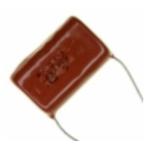
ECQ-P4394JU Panasonic Electronic Components CAP FILM 0.39UF 5% 400VDC RADIAL
