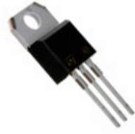
TYN812TRG STMicroelectronics SCR 12A 15MA 800V TO-220AB
