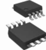
DS1050U-025+ Maxim Integrated IC OSC PROG TIMER 25KHZ 8USOP
