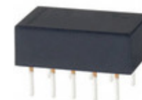
TQ2-5V Panasonic Electric Works RELAY TELECOM DPDT 1A 5V
