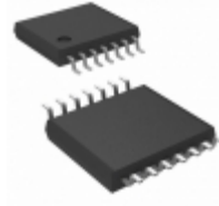
MM74HCU04MTCX Fairchild/ON Semiconductor IC HEX INVERTER UNBUFF 14TSSOP
