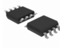
BR24G64FJ-3AGTE2 Rohm Semiconductor IC EEPROM 64KBIT 1MHZ 8SOP
