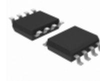
BR24G64F-3AGTE2 Rohm Semiconductor IC EEPROM 64KBIT 1MHZ 8SOP
